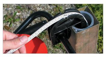
A Tape Guide allows depth measurements to be read at the marked position on the Tape Guide, to give reliable, repeatable, accurate depth measurements when profiling a well. The Tape Guide protects the tape from damage on rough edges of well casing.
